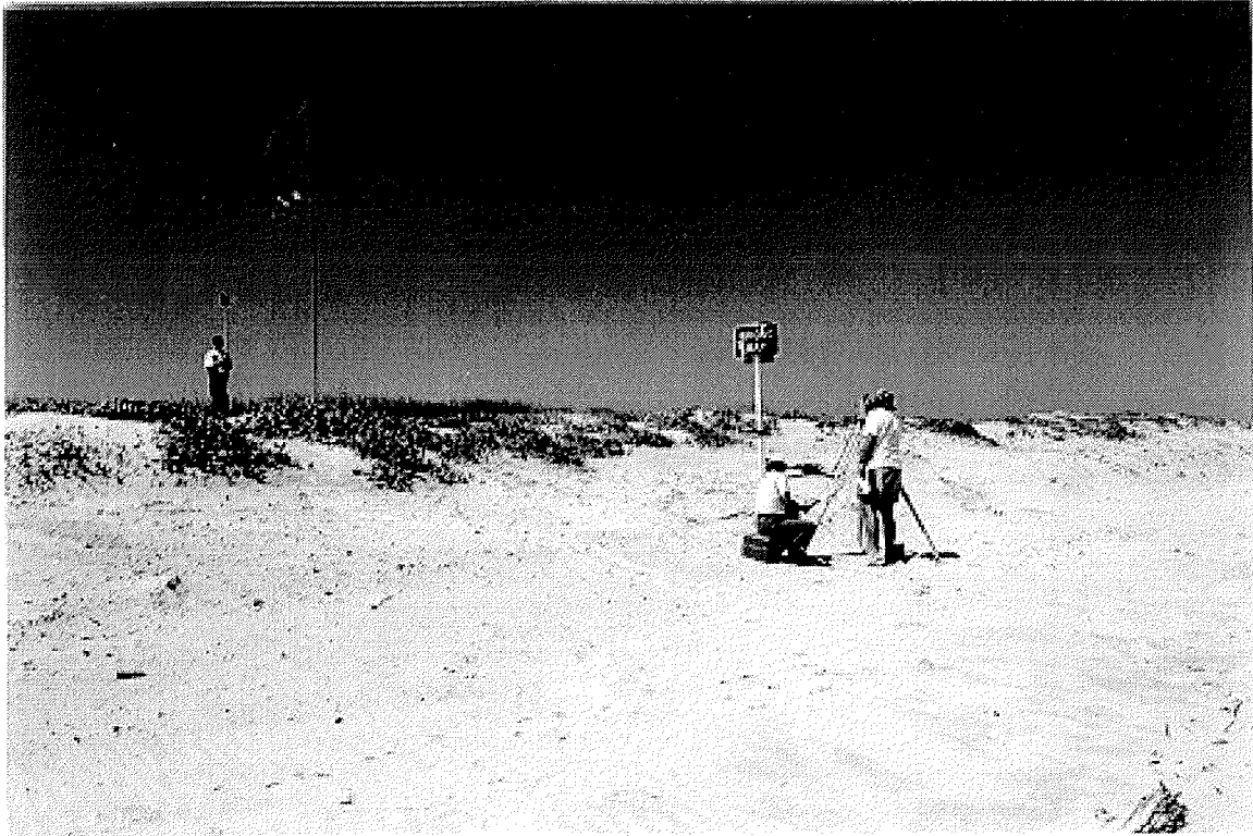
Figure E5. Land portion of beach profile survey.
